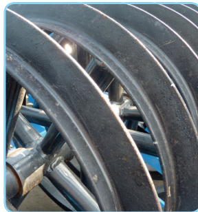
T-ring roller \phi 600 mm / T-Ring Walze \phi 600 mm / Rouleau T-RING \phi 600 mm
